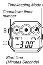
With the countdown timer, you can set up to nine start times, which are counted down in sequence one after the other.
